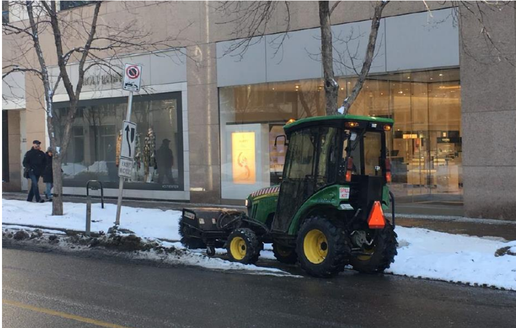
Example of a John Deere tractor from the City of Calgary clearing snow in a protected bike lane. This tractor has different attachments (brush, bucket, sprayer on the back) that can be used to clear snow, leaves, and other debris from a cycling facility.
