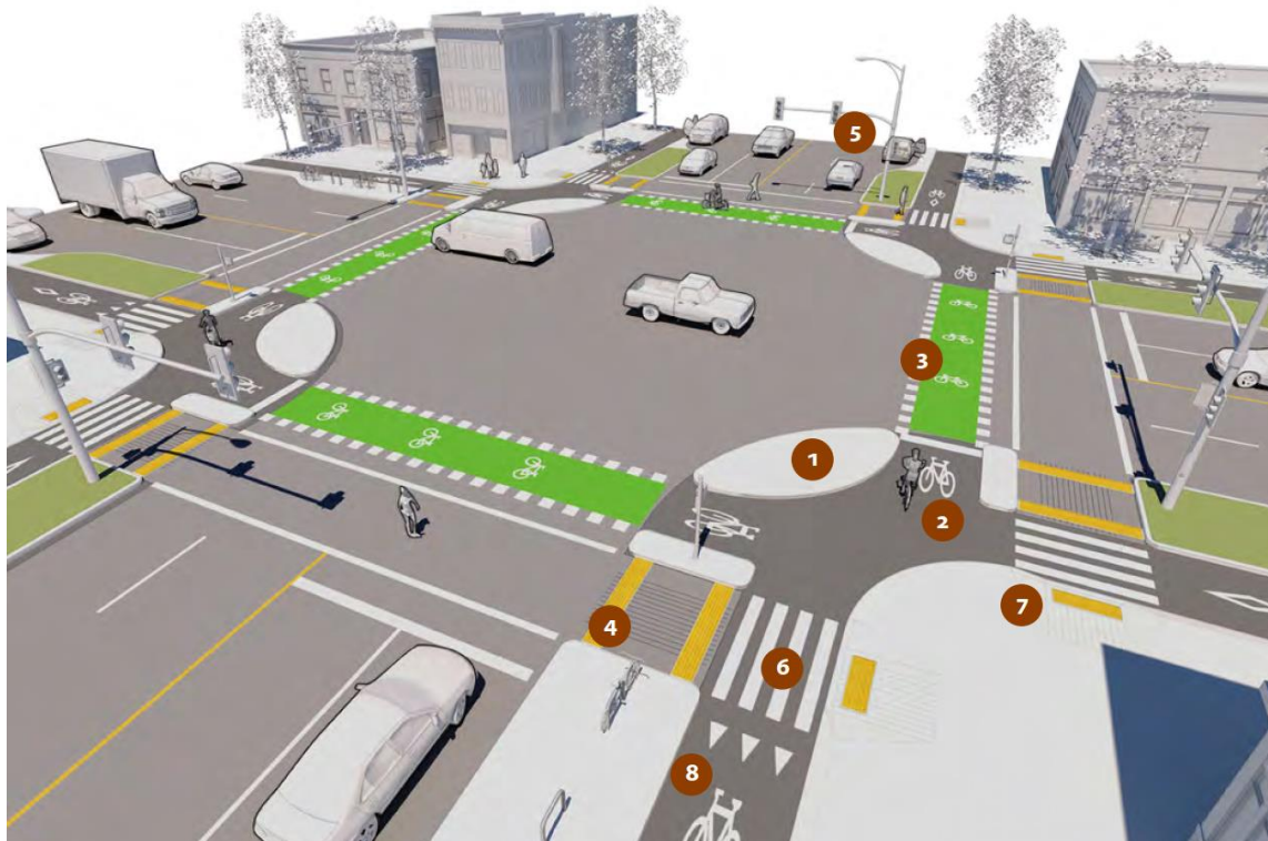
Important elements to be considered as part of protected intersection design. Numbering reflects list of design elements below. Image retrieved from Figure G-90 of the BC AT Design Guide (2019).
